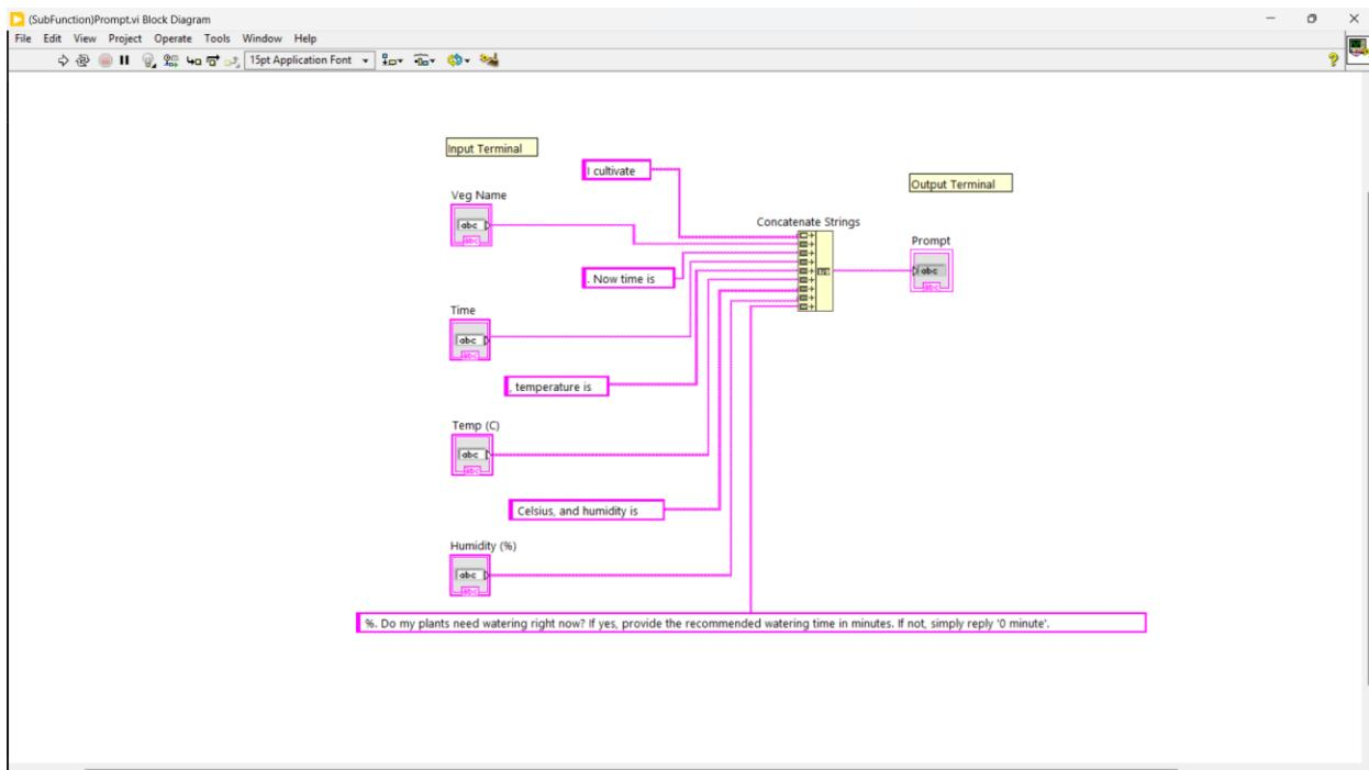
This LabVIEW module generates a dynamic text prompt based on current environmental and crop-specific inputs to assist in automated decision-making, typically by an AI or chatbot system. It takes inputs such as the vegetable name, current time, temperature, and humidity, and uses the Concatenate Strings function to assemble them into a complete, context-rich sentence.
