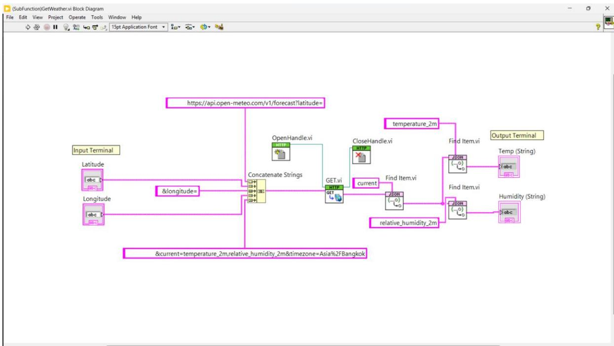
This LabVIEW module is designed to fetch real-time weather data—specifically temperature and humidity—using the Open-Meteo API. It takes latitude and longitude as inputs from the user, constructs a URL by concatenating the necessary parameters, and performs an HTTP GET request using built-in VI functions ([OpenHandle.vi](#), [GET.vi](#), and [CloseHandle.vi](#)) to retrieve live weather information.
