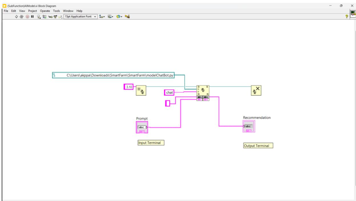
This module is part of the main system and integrates an AI-powered chatbot to provide real-time recommendations and responses based on user input. The system uses a Python script (ChatBot.py) executed via LabVIEW to handle AI processing, making the solution both flexible and scalable.
