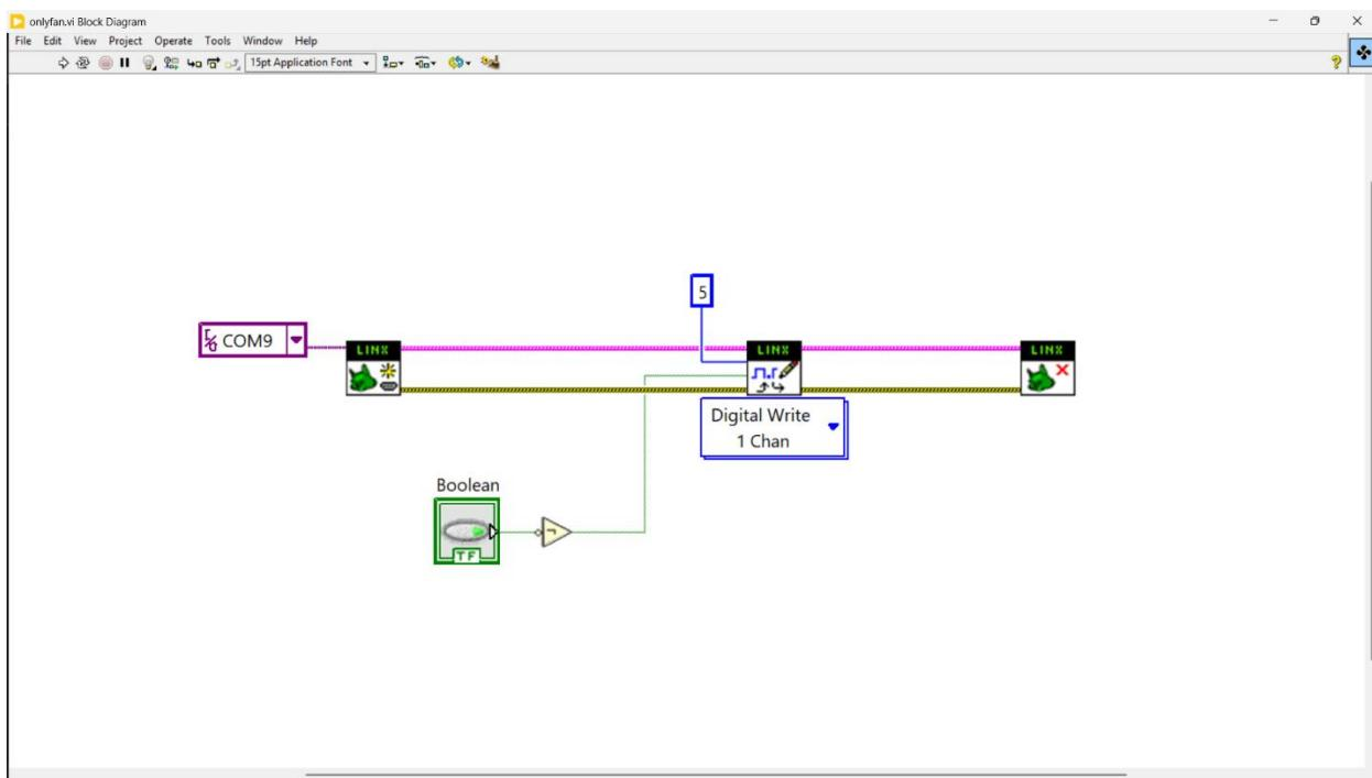
This VI establishes communication with an external microcontroller via the COM9 serial port using the LINX toolkit. It uses a digital output channel ([pin 5](#)) to control a fan. When the Boolean switch is toggled to True, the logic signal is inverted and sent to the Digital Write block, activating the fan by setting the pin LOW (assuming active-low logic).
