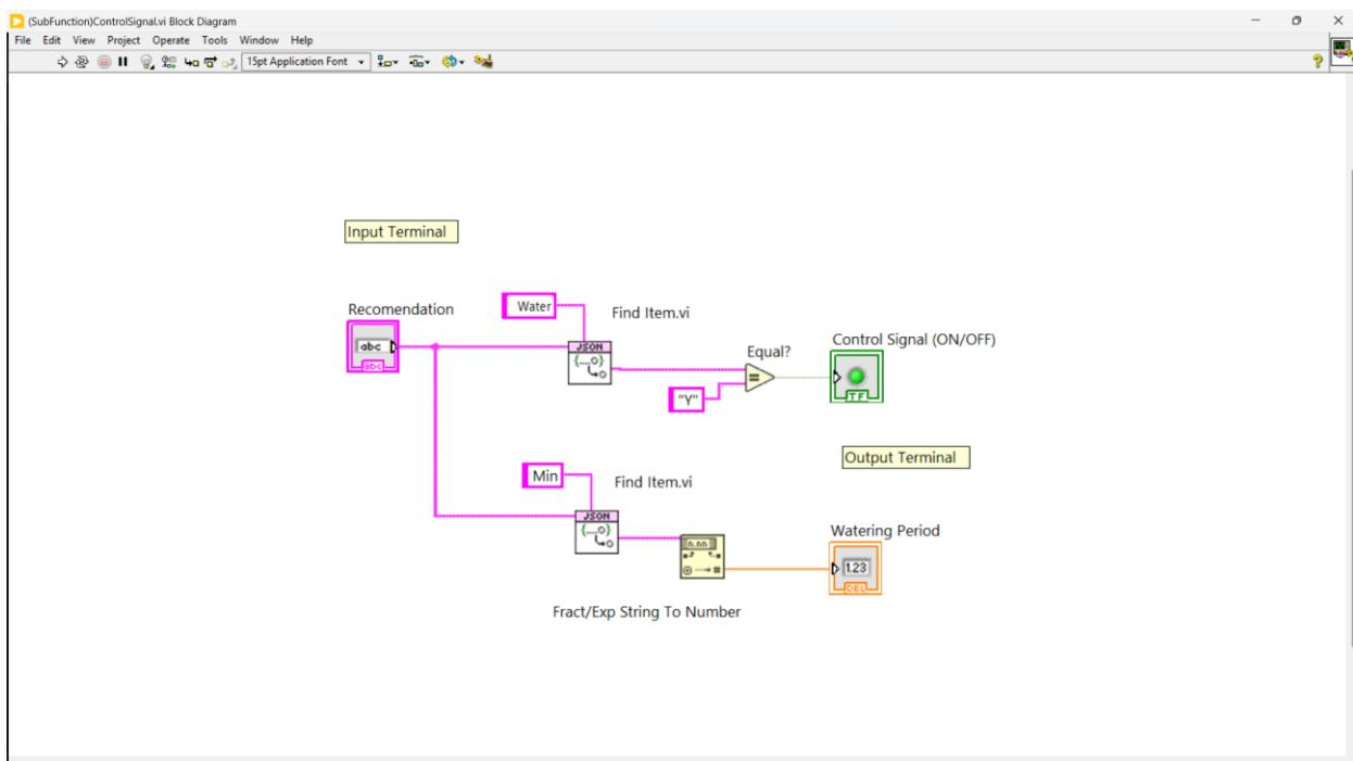
This module is part of an automated irrigation control system, designed to manage plant watering recommendations based on predefined conditions. It interprets textual commands and activates a control signal to initiate watering when specific criteria are met.
