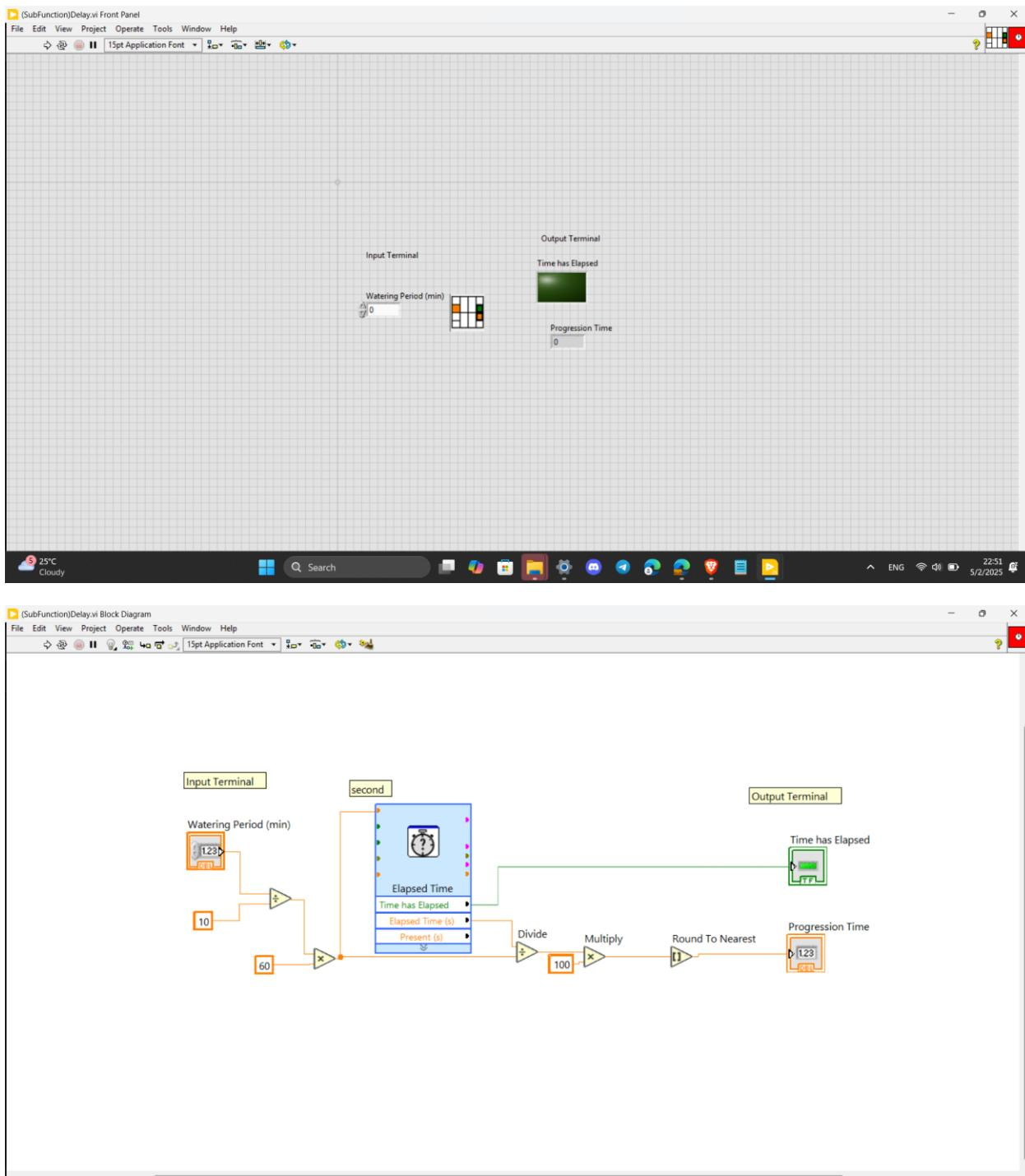
This section of the main system implements a timer function to manage and monitor the watering period within the overall irrigation control system. The user inputs the desired watering period in minutes, and the system tracks elapsed time in real-time to determine when watering should stop.
