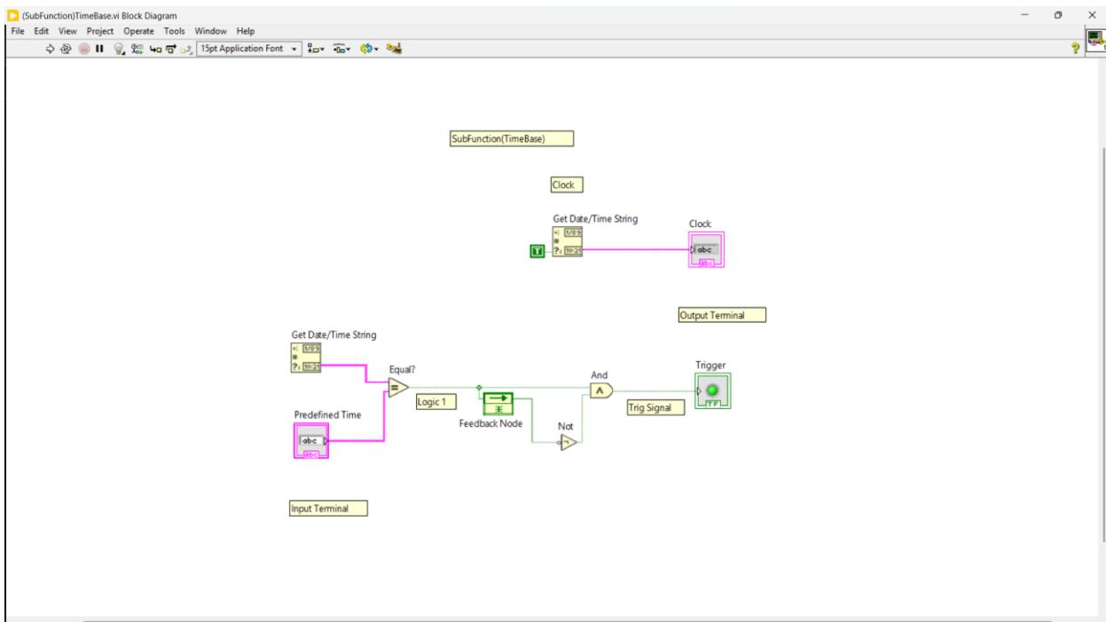
This module implements a time-based trigger mechanism that activates specific actions at a predefined time. It continuously reads the system's current time using the Get Date/Time String function and compares it with a user-defined time input. If the current time matches the predefined value, a logic block evaluates the condition, and a trigger signal is generated accordingly.
