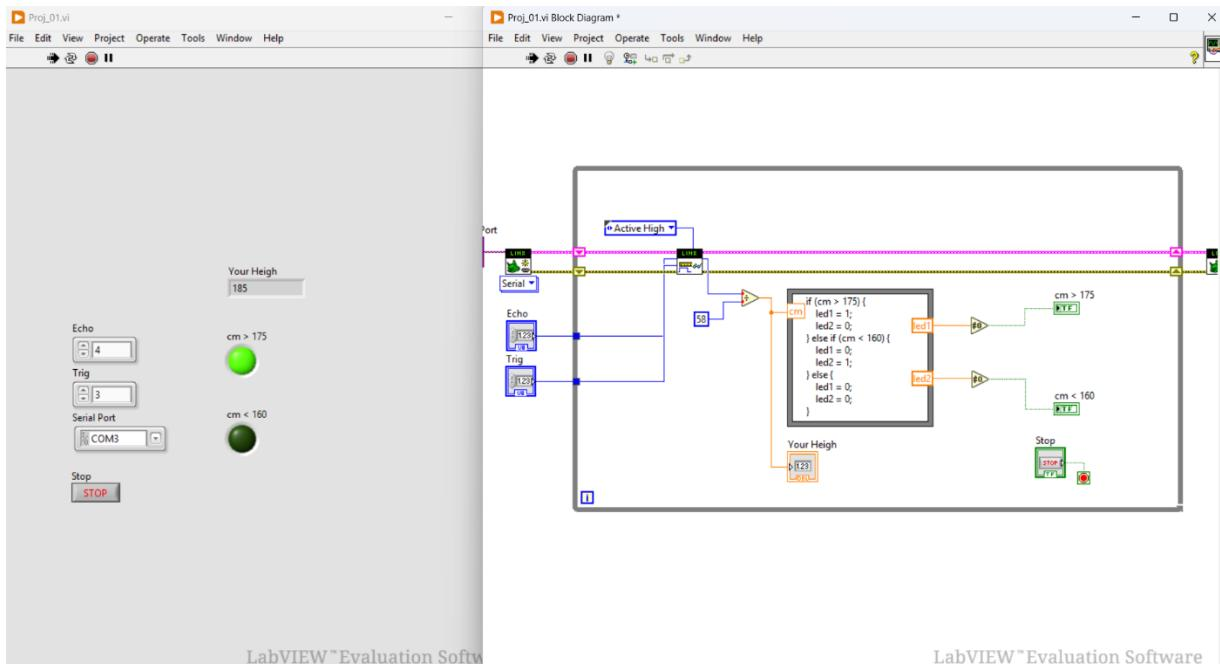
This project presents a height measurement device using an ultrasonic sensor integrated with LabVIEW software. The ultrasonic sensor measures the distance from the sensor to the top of a person's head by sending and receiving ultrasonic pulses. The time taken for the echo to return is converted into centimeters, giving accurate reading.
